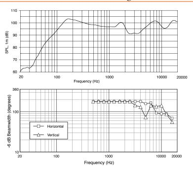
Frequency Response, on axis in half-space, 70V input to 25W tap
