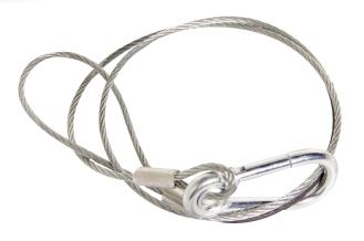
Weight: 0.1 lb (0.04 kg) Load Capacity: 60 lb (25 kg) Length: 31 in (787 mm)
