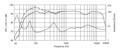
Frequency Response, on axis in half-space  $(2\pi, dotted)$ line) and full space ( $4\pi$ , solid line) at thru ( $4\Omega$ ) setting, Input Impedance.
