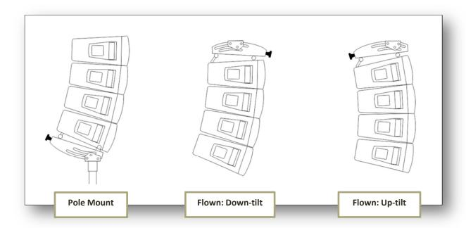
Note that there is only one orientation for pole mounting the MLA Mini. You should not under any circumstances attempt to pole-mount MLA Mini with an up-tilt, this will be unsafe.
