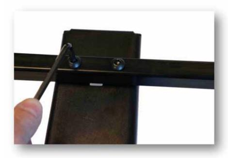
First attach the front arm to the two M8 Inserts on the top of the arc bracket using the two M8 x 35mm button head screws and the M8 washers. This must be fitted to the two insets furthest from the angle adjustment knob. Tighten these using the 5mm Allen Key (not supplied). Note the orientation of the cross arm, in all modes of operation the cross arm must be fitted with the single tabs at each end upwards and the double slot downwards.
