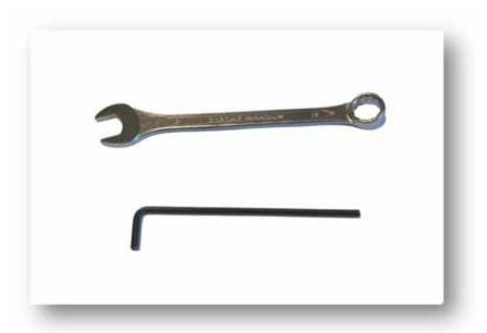
The principal tool required for assembly of the bracket is a 5mm Allen Key used to fit the front arm and the swing arm bracket. For fitting the ASF20045 pole mount adaptor or scaffold clamps, a 19mm (3/4") spanner (wrench) will be required. (Tools are not supplied)
