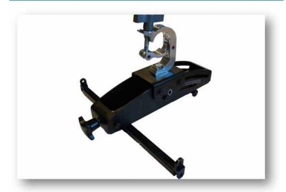
The Universal Bracket is used inverted for flying applications. The front arm must therefore be attached as for pole mounting but the opposite way up. For down-tilt applications it will need to be attached to the end closest to the angle adjustment knob. Note the orientation of the tabs on the front arm. This must remain with the single tabs facing upwards and the double slots facing down.
