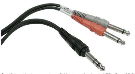
Send Return (also known as a Insert Cable), conventionally wired: TIP = Send, RING = Return. Can be used as a "Y" to split stereo signal into Left and Right. In this case, Right = RING and Left = TIP.
