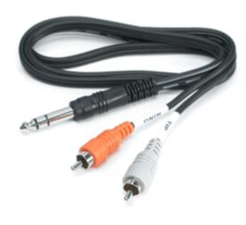
Send Return (also known as a Insert Cable), conventionally wired: TIP = Send, RING = Return. Can be used as a "Y" to split stereo signal into Left and Right. In this case, Right = RING and Left = TIP.
