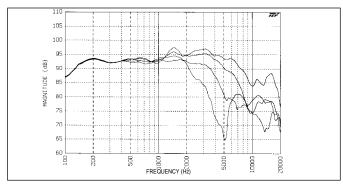
C10A: Fundamental vs 2nd & 3rd Harmonic (Raised 20dB)@ 1 watt
