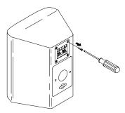
Step 2 – Loosen nut on the outside of the MTC-PC2. Run wire through the gland fitting, as shown. Do NOT tighten the nut on the outside of the MTC-PC2 yet.
