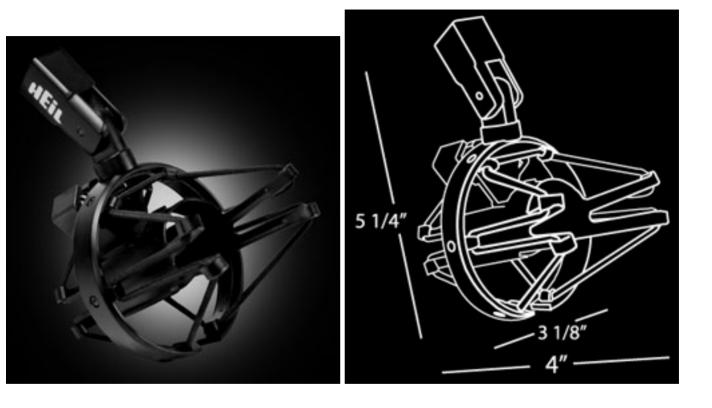
The SM-1 Shock Mount is an 8-point flexible suspension support system that helps suppress low-frequency rumble on the microphone line by absorbing and damping vibrations picked up from the studio desk or console.
