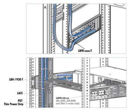
Allows vertical and horizontal cable management.
