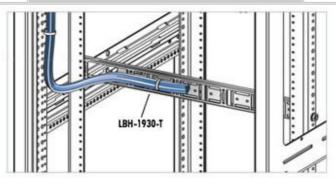
A complete cable management system, the NEW telescoping lacer bars adjust to fit any Middle Atlantic Products rack.
