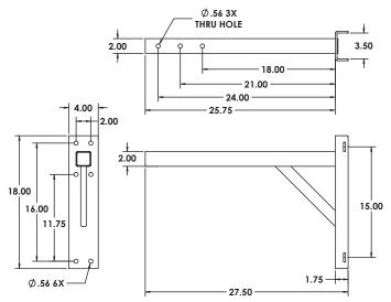
May be used with dual adapter for a 3-way speaker installtion Comes with Band Kit, for poles up to 25" in diameter
